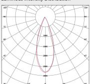
Luminous intensity (cd/klm) in level C 0° – 180° Luminous intensity (cd/klm) in level C 90° – 270°
