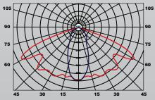
Luminous intensity (cd/klm) in level C 0° – 180° Luminous intensity (cd/klm) in level C 90° – 270°
