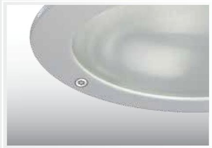
**Body :** made of Galvanized Steel with the frame made of high pressure die-cast aluminum alloy finished to corrosion class II by high pressure to spraying at 2.5 bar before its finally electro-statically powder coated with a 60 micron thermo-hardened polyester powder, stabilized and UV protected.
